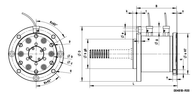
The quill shaft geometry and composition is dependent on customer requirements.
